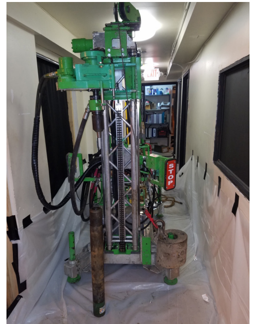
Explor 220 Electric Geotechnical Drill Rig
