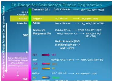
Figure 19 - EH Range for Chlorinated Ethene Degradation
