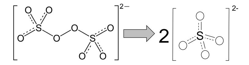
Under thermally activated conditions (i.e., temperature of 40~100°C), there is considerable evidence that the persulfate anion can be converted to a powerful oxidant known as the sulfate free radical which could be used in situ to destroy HVOC contaminants in groundwater and sorbed to the soil matrix.
