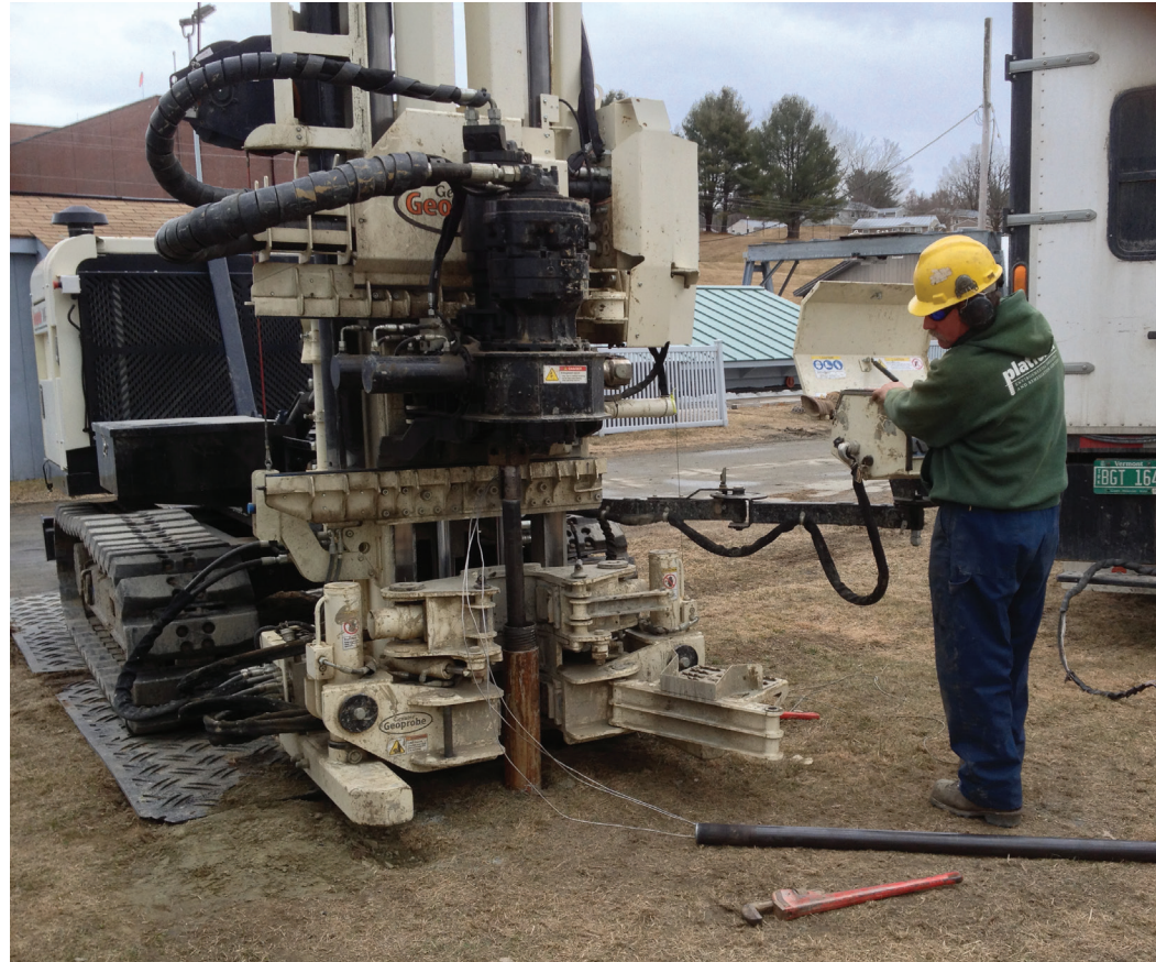
Contractors can overcome DPT refusal, but solutions can introduce safety concerns that may not have been previously planned for. Source: Cascade Environmental photos
