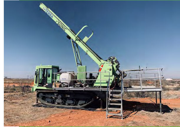
New Tsi 150C sonic drill rig
