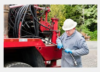
Hydraulic hose inspection is critical in preventing leaks and broken hoses
